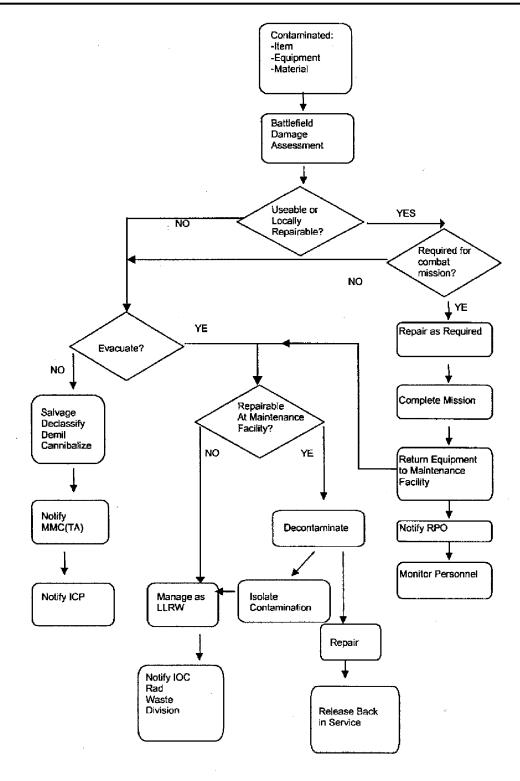
Figure 2-1. Flow Chart for Retrograde Material Condition 1
